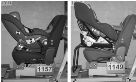
Pictures of a RF US design with flexible lower webbing, and a RF European design with rigid ISOFIX connectors and support leg.
